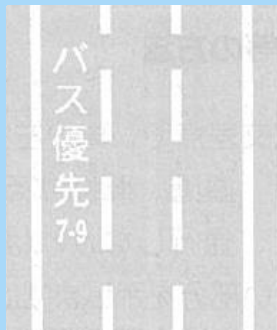
Letters marked on lane indicates priority lane for buses during the period indicated. Other vehicles may use but must not interfere with the bus traffic.
