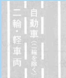
Letters marked on lanes indicate order of travel. Letters at the left indicate EXCLUSIVE use of two-wheel vehicles and light vehicles. Letters at the right indicate EXCLUSIVE use of motor vehicles except two-wheel vehicles.
