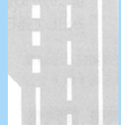
Large white dotted line is used for most outer line near the entrance of the National Motor Vehicle Expressways.
