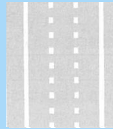
A solid white line for most outer lane, combined with dotted lines using metal and/or reflective "Buttons" also indicates line dividers.
